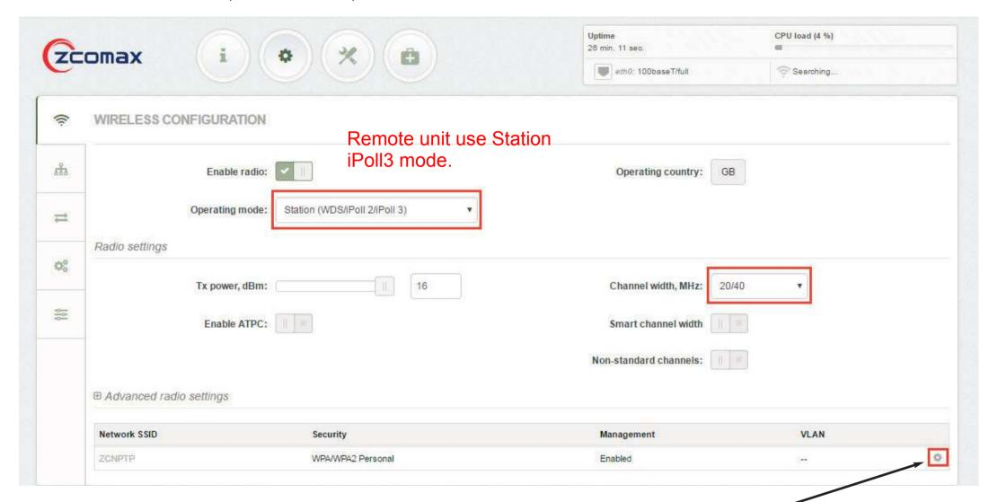
Click on the right hand side button in Wireless settings (AP) section to change SSID and Encryption configuration.
